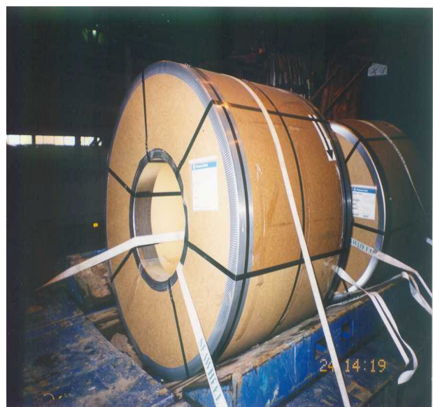
Straps through and across the coil
