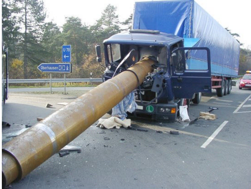
Picture 1: During heavy braking, the badly secured steel tubes made their way through the headboard and the drivers cab.
