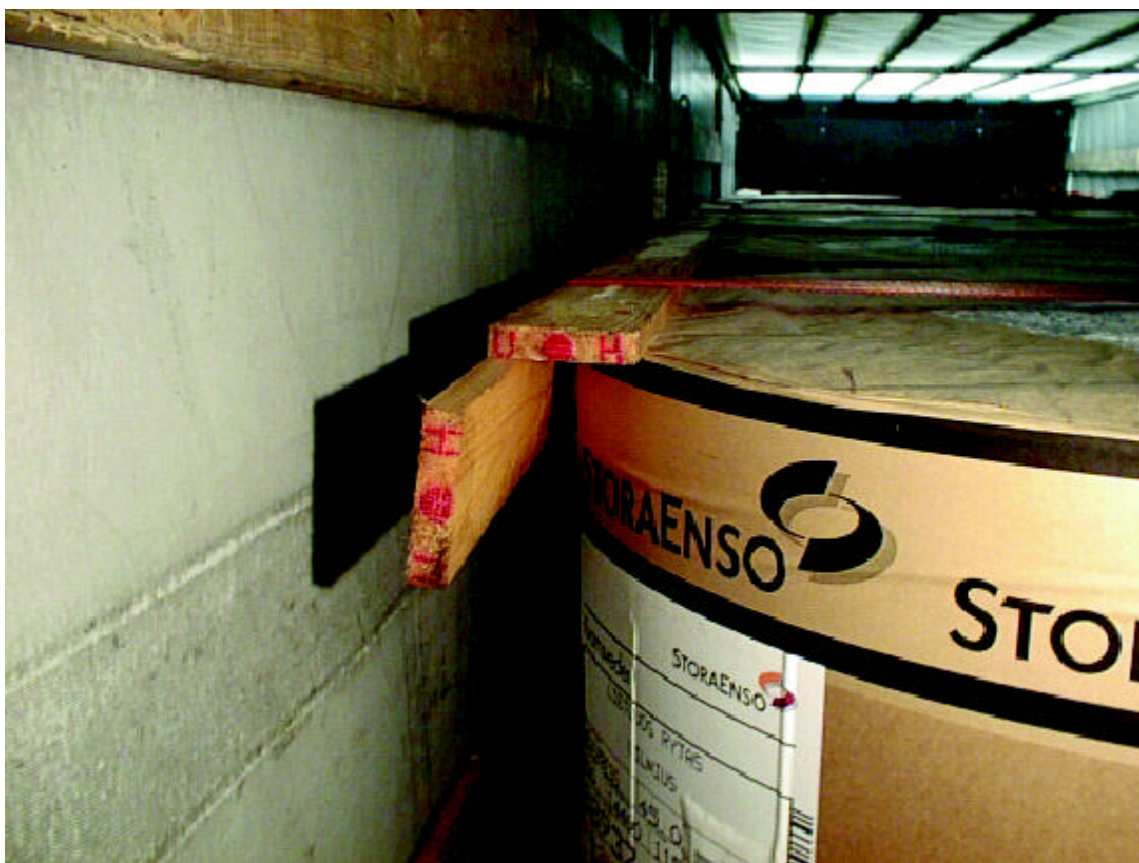
Picture 53: Edge beam made of wooden boards.
