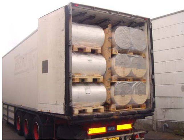
Picture 18: Filler between the rows of cargo
