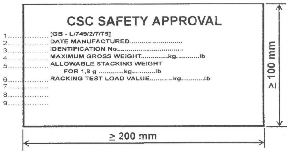
Figure 8.10.7-4: Safety approval plate on container
