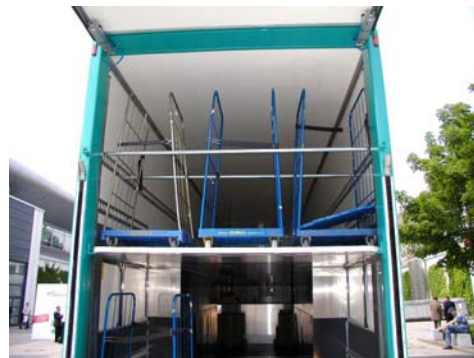
Picture 64: Wheel pallet with side supports and clipping bars
