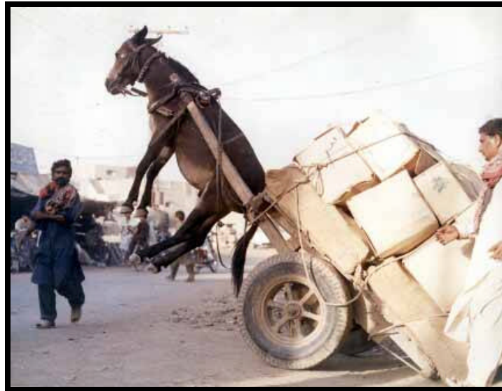
Picture 5: Incorrect load distribution. Funny things might happen...or it can have dramatic results.
