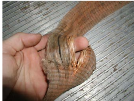
Picture 36: Severely damaged webbing? Throw it in the waste basket!
