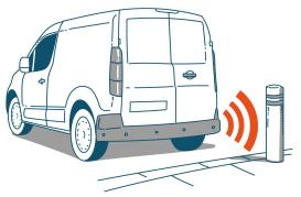
Reversing and parking aids minimise the chances of damage, injury, or prosecution. They can detect obstructions around the vehicle in the driver's blind spot such as bollards, pedestrians and other vehicles.
